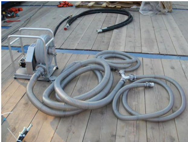
Figure 19 Hydraulic Air Blower HAB 200 and air hoses
