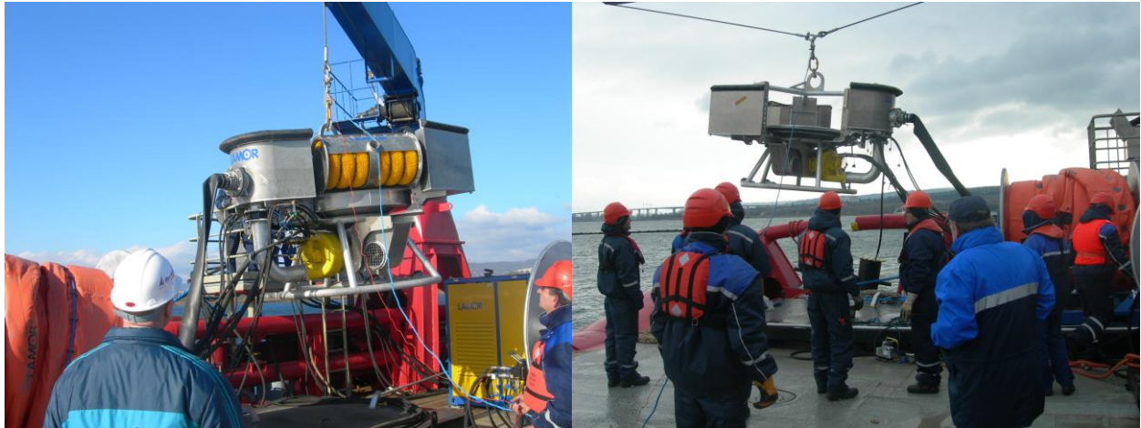
Figure 12 – Weir Skimmer LWS 1300 Mk II with brush and weir modules
