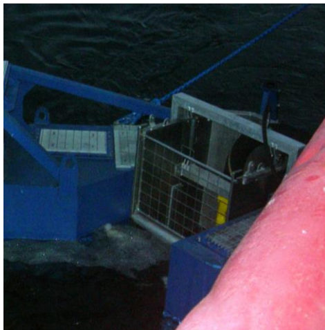
Figure 3 LAMOR Stiff Sweeping Arm LSS 15m – weir skimmer module
