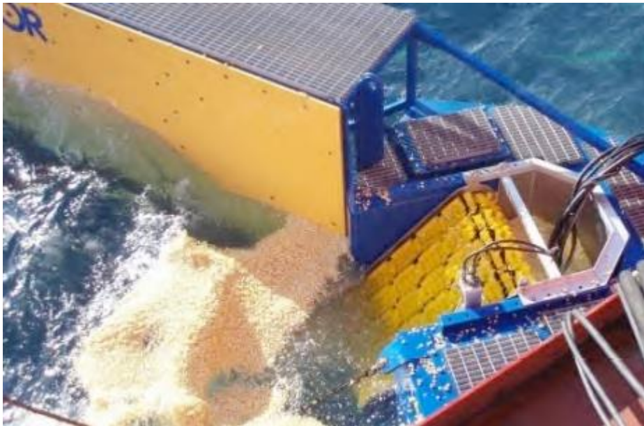
Figure 5 LAMOR Stiff Sweeping Arm LSS 15m – brush skimmer module
